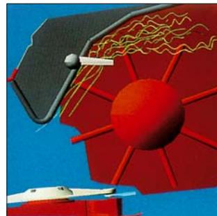
As crop flows between the comb teeth, the natural wax coating is opened along the length of the stem, allowing maximum moisture content to evaporate.
