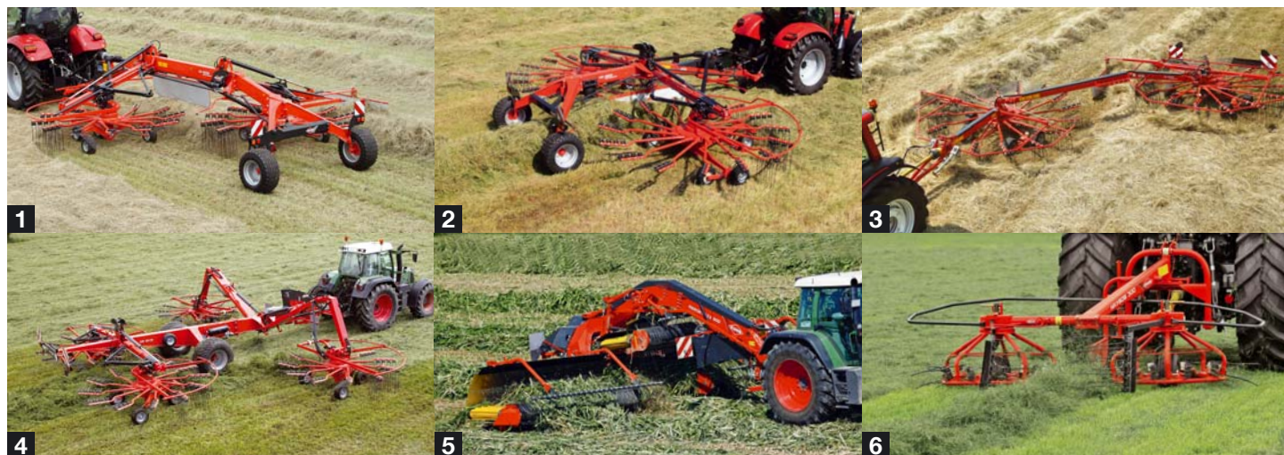
1. Semi-mounted twin Gyorakes with side delivery - 2. Semi-mounted twin Gyorakes with central delivery - 3. Trailed twin Gyorakes - 4. Four-rotor Gyorakes - 5. Belt mergers - 6. Tedder-rake combinations
