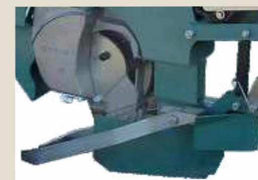
Assolcatore a falcone in ghisa speciale Shoe type furrow opener made in special cast iron
